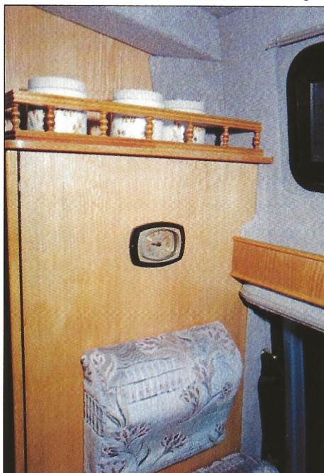
Clock, gallery rail and side trough for occasional storage.
